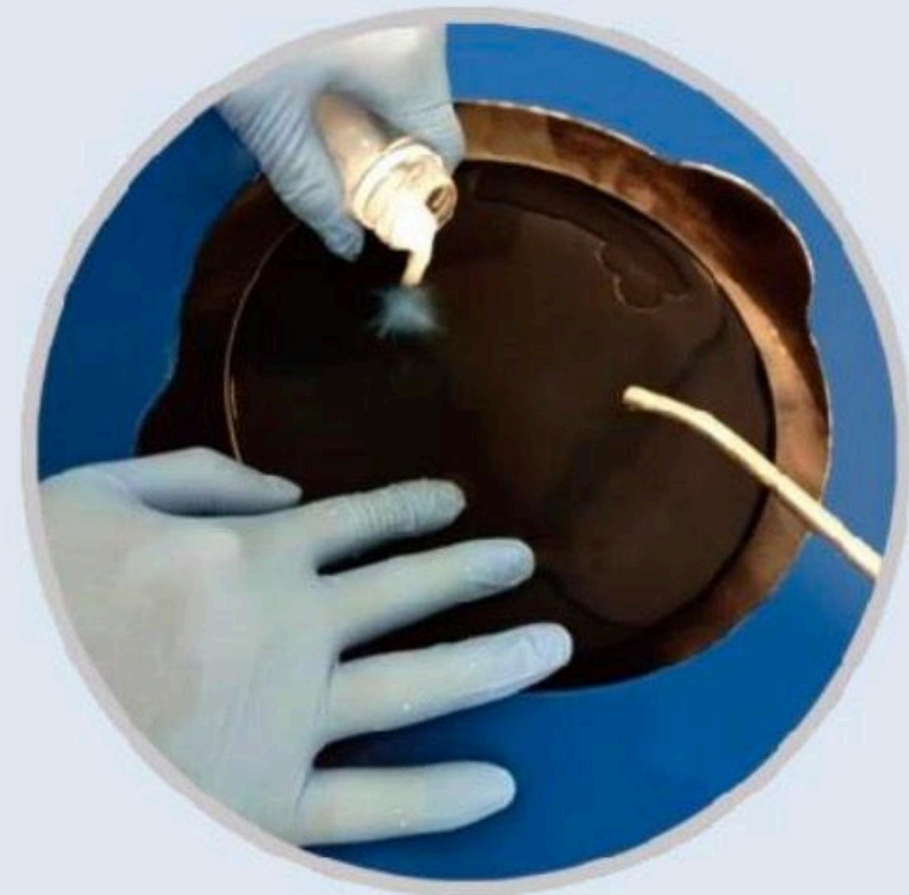
English: Perform fixed-point or non-fixed-point grinding, combined with the use of Ion Milling, to achieve a clearer cross-sectional effect.
